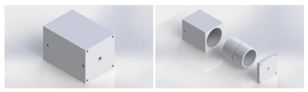
The low pressure cylinder receives partially expanded steam from the high pressure cylinder. Timing is dependent on the timing of the high pressure cylinder, so no valves are required. Steam expands for its second stage before exiting through the uniflow exhaust.
