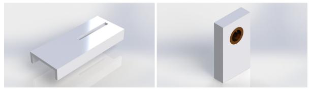
The base (left) is where all of the components are mounted and holds them in the correct orientation. The two support bearings (right) mount to the base and hold the crankshaft in place.
