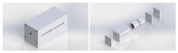
The high pressure cylinder is where the first stage of expansion occurs. A steam reservoir is supplied to the bash valves which regulate inlet timing. Due to the geometry constraints of a mechanical bash valve, the valve must be open before dead center for the same amount of time that it is open after dead center. Exhaust occurs through two separate uniflow ports (one for each side of the piston) which connect to corresponding inlets on the low pressure cylinder.
