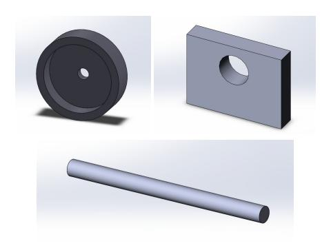
The Shaft assembly consists of a shaft cylinder, shaft mounts, bearings and a flywheel. There were two shaft mounts placed on the base plate, one in front of the flywheel and the other in front of the trilobe cam and behind the inlet cam. The shaft cylinder was placed through both mounts, flywheel, and through the cams, up to the trilobe cam. The adjustments were made to the
