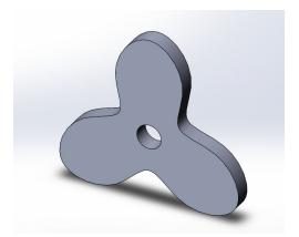
The Trilobe cam is where the linear motion from the pistons is converted into rotational motion for power generation. No changes were made to the Trilobe cam. There have been considerations in previous designs for different shapes such as an asymmetrical trilobe cam or a tristar cam, yet the Trilobe Cam was considered to be better.
