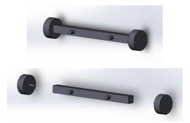
The Piston assembly consists of a piston rod and two piston pins. The piston rod has two pins sticking out for bearings that would move the trilobe cam. No changes were made to the design from the first versions. Some future additions could be the addition of a system where the bearing pins could be spring loaded to add some tolerance to the piston-trilobe mechanism.
