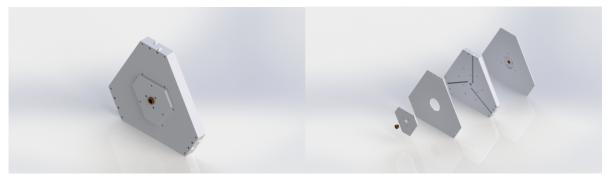
The main plate has 3 manifolds on each side to pass exhaust and inlet steam to and from the cylinders. On each side of the main plate are additional thin plates that cover the milled manifolds and house the disk valves. One last plate on each side covers the disk valves, supports the bronze bushings, and has ports for inlet and exhaust.
