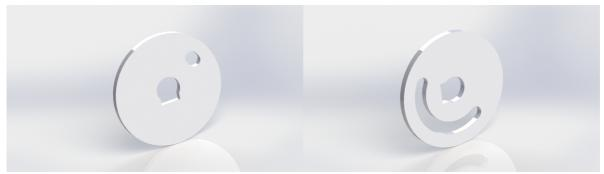
Both the inlet disk valve (left) and the exhaust disk valve (right) have a center hole with a keyway for the shaft and key to run through. The length and positions of the curved slots determine valve timing.
