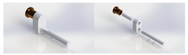
The crankshaft has a large overhung crank that is responsible for turning all 3 pistons. Since the crank drives all 3 pistons, it is subject to significant forces and must be relatively thick to compensate. A bushing sleeve is fit over the crank pin so the piston rods can rotate smoothly. On the shaft, there are 2 flats which hold the keys that line up with the corresponding disk valves and hold them in place.
