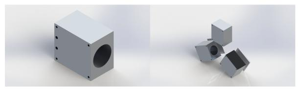
The cylinder blocks are separate for each piston and have 2 holes at the head for inlet and exhaust. Spacers are added between 2 of the cylinder blocks and the backing plate so that each cylinder is slightly offset and all 3 piston rods can attach to the same crank without interfering with each other.
