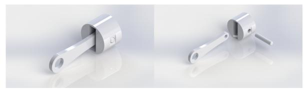
The piston consists of the piston head, piston pin, and piston rod. The pin is press-fit to the rod, but given clearance through the head. The pin stays in place by slight contact with the cylinder wall on each side. In this way, the rod is free to rotate along the axis of the pin, but held in place otherwise.
