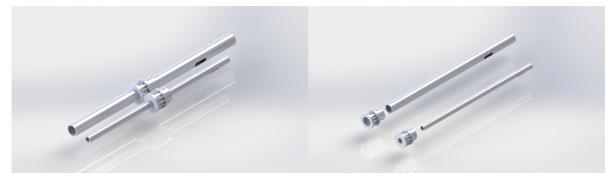
The valve pipes have 2 slotted cuts that line up with each cylinder manifold and are diametrically opposed from each other. Since they are hollow, the pulleys are attached on the ends with 2 set screws. The pulleys hold a belt which connects between the two valve pipes and the crankshaft.
