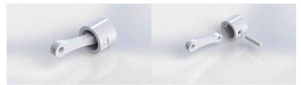
The piston consists of the piston head, piston pin, and piston rod. The pin is press-fit to the rod, but given clearance through the head. The pin stays in place by slight contact with the cylinder wall on each side. In this way, the rod is free to rotate along the axis of the pin, but held in place otherwise.
