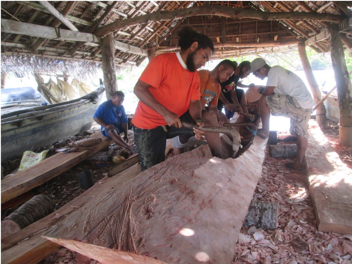
Fine carving keel in Lamotrek canoehouse after seasoning. Isayah Yarofayan in foreground. Photo – Isayah Yarofayan
