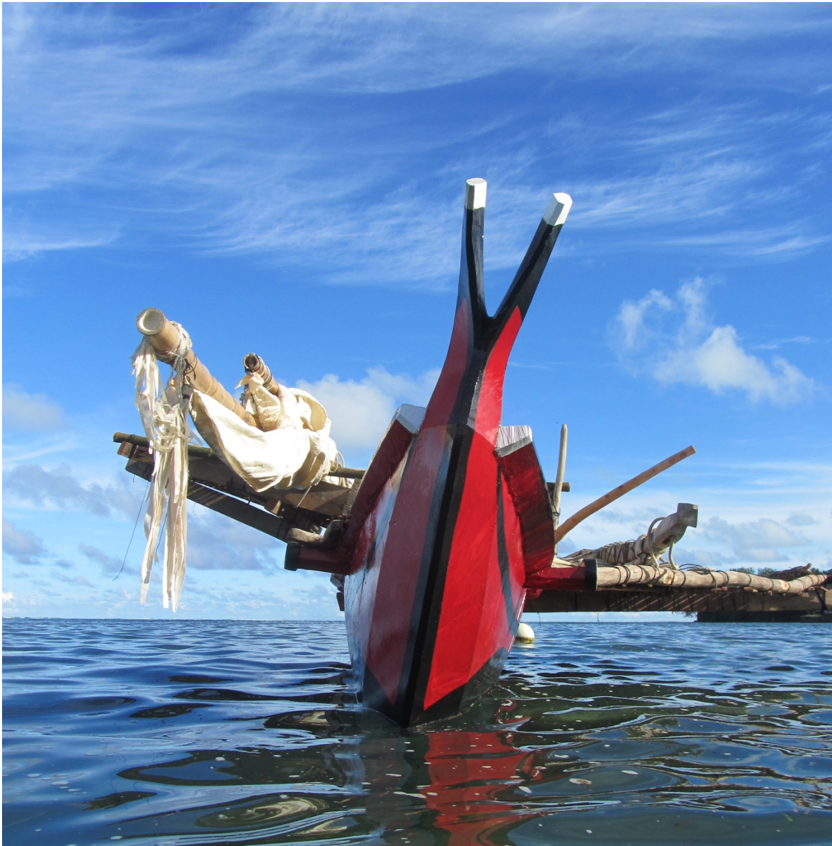
Mathou Maram II hull showing asymmetry and scalloped chines. Photo- author
